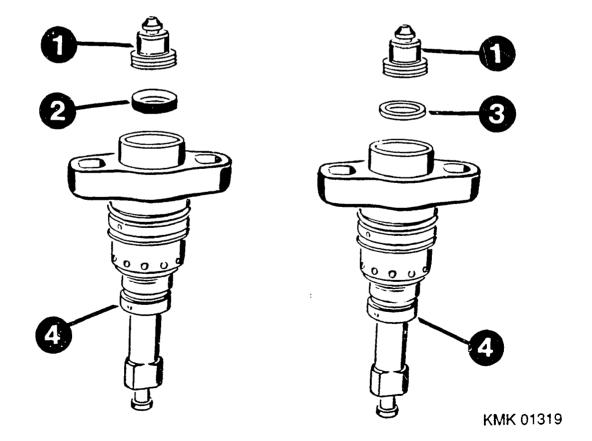
Sealing caps are additionally contained in the parts set 2 417 010 010 as of date of manufacture 166.
